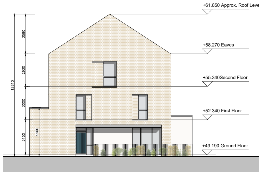
DUPLEX BLOCK N SIDE ELEVATION (NORTH)
