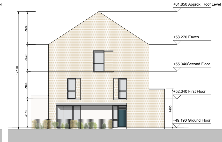
DUPLEX BLOCK N SIDE ELEVATION (SOUTH)
